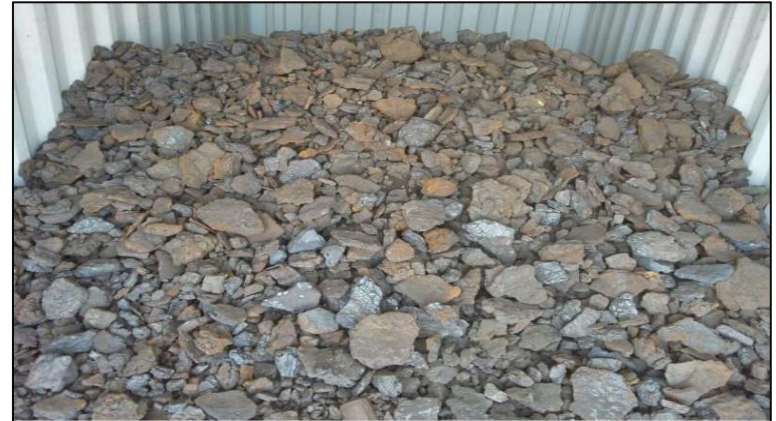
Iron Slag (Waste Material of Steel Industry)
